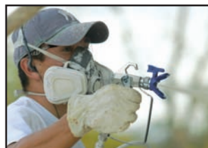
New FTx 4-finger gun trigger – full length trigger is easier to hold in continuous spray.
